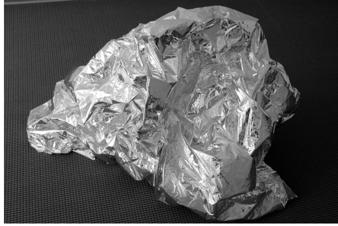
Figure 1.5: A loosely crumpled sheet of aluminised Mylar, 2 metres in width and 10 microns in thickness [26].
